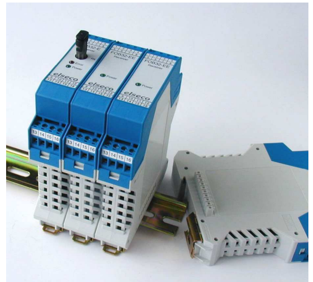
Receiver FOB32-EGG (Master) and 3 FOB32-EEG (Slaves)
